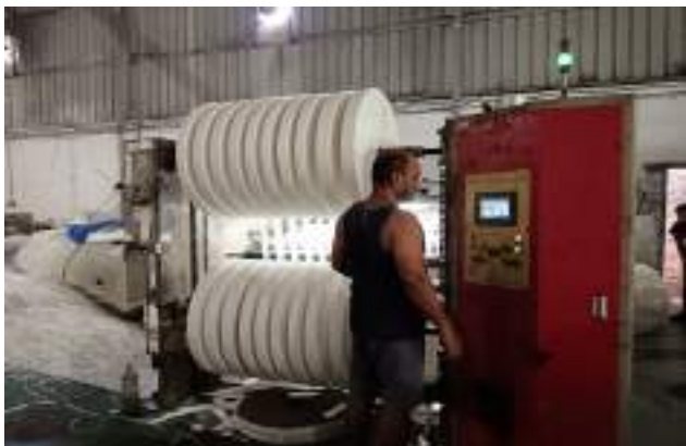
Slitting Reels into 'Bobbins'
