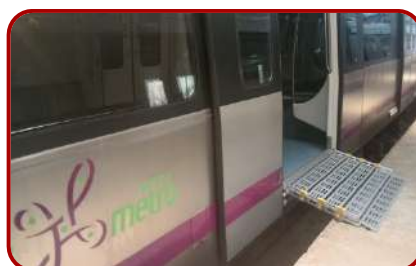
Emergency Evacuation Ramp
